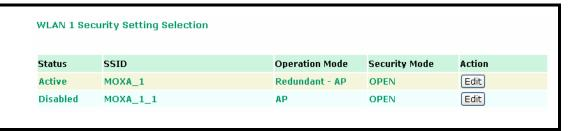
The AWK-5222 provides four standardized wireless security modes: Open, WEP (Wired Equivalent Privacy), WPA (Wi-Fi Protected Access) and WPA2. Several types of security models are available in AWK-5222 by selecting *Security mode* and *WPA type*:
