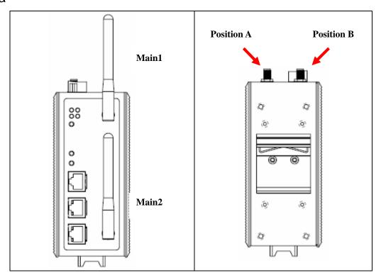
If you need to improve the performance of the Main1 and Main2 antennas, you can connect additional antennas to the side panel of the AWK-5222 using an antenna cable (Position A: AUX1 and Position B: AUX2). The default antenna for the AWK-5222 is a 2 dBi, dual-band omni-directional antenna, RP-SMA (male).
