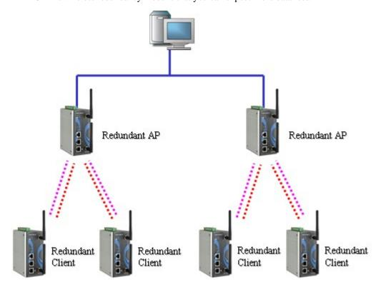
The following figure shows the Wireless Redundancy operation mode:
